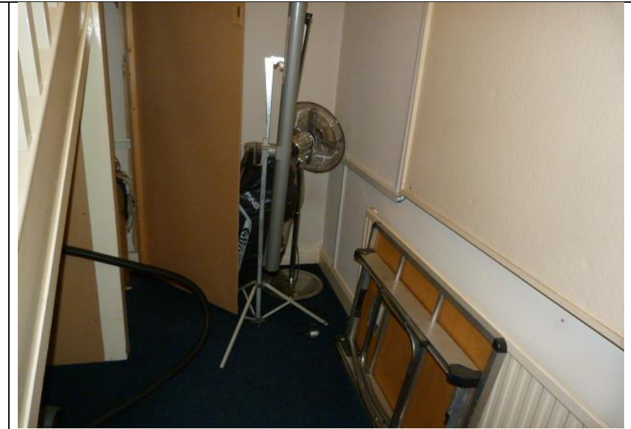
Item 55 Combustibles including electrical items located under the Town Council staircase Priority: Medium
